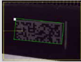
Low-contrast code Code is made legible through high tolerance – also towards weakly contrasting codes.
