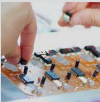
Checking accuracy of installation or presence of components
