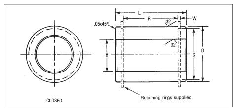
Material: Self Lubricated Engineered Plastic
