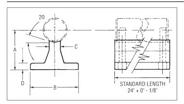
These rails are supplied without mounting holes and can be used horizontally or vertically to provide optimum rigidity (see pre-drilled aluminum rails for sizes and specifications). Shaft support rails are available in standard lengths of 24'' + 0'', -1/8 (600 + 0, -3.2 mm), but can be supplied to meet shorter length requirements or placed end to end to meet longer length requirements.
