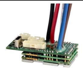
The **FM060-25-RM** is a single-axis servo drive and integration board assembly for a FE060-25-RM FlexPro<sup>®</sup> series servo drive with IMPACT<sup>TM</sup> architecture. Connections to the controller, motor, power, and feedback are simplified through the standard connectors featured on the board.
