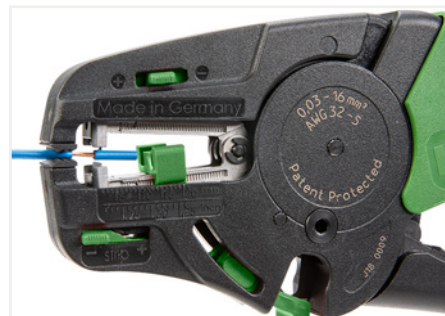
Partially stripping a conductor.
