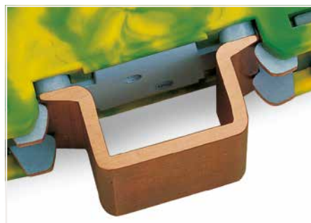
Grounding foot: Ground conductor terminal blocks (limited to max. 120 mm 2 /250 kcmil per EN 60947-7-2) must be snapped onto a 2.3 mm thick copper DIN-rail.
