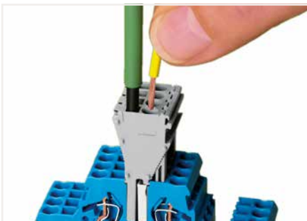
CAGE CLAMP® termination: Tap-off modules are used when additional or removable connections are required (can be used as a permanent connection or a test plug). Wiring is possible whether the modules are plugged into the assembly or not.
