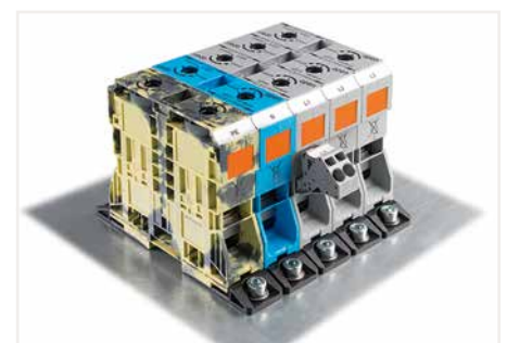
Secure the terminal block to a mounting plate using two M8 cylinder-head screws and appropriate washers.
