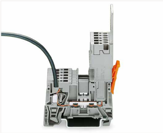
1-conductor female plug Carrier terminal blocks can be commoned via 280 and 780 Series Jumpers and tested using a test plug adapter (280-4..).
