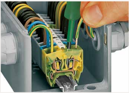
CAGE CLAMP® termination: Inserting a conductor. With ferruled conductors, it is necessary to use a terminal block one size smaller than the conductor's nominal cross section.
