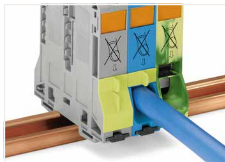
Yellow, detachable finger guards provide touch-proof safety by shielding jumper contact slots and/or unused conductor entries.
