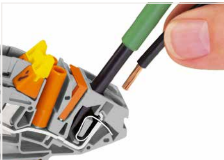
CAGE CLAMP® connection Inserting a conductor.
