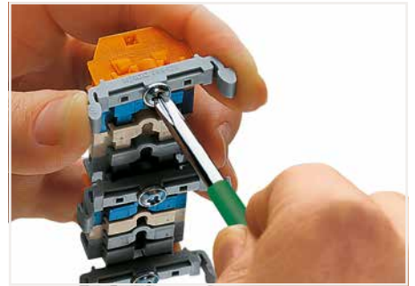
Mounting and securing a terminal strip directly to the plate via screw-type flanges. screwing a mounting foot (209-123) (distance between mounting feet: approx. 20 ... 25 mm)
