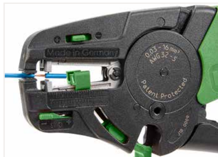
Partially stripping a conductor.
