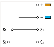
Sensor terminal block
