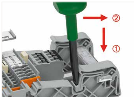
Release the mounting bracket by pushing the operating tool down ① and then forward ②.
