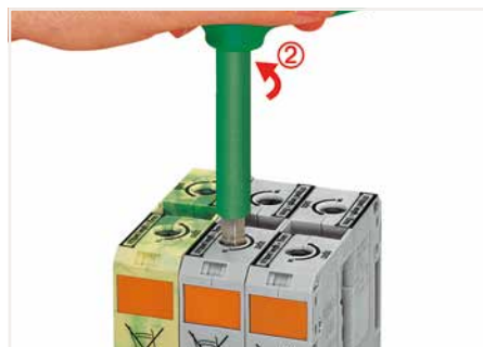
Conductor termination – step 3: A short counter-clockwise rotation ② releases the tab. When unlocked, the T-wrench rotates clockwise, securely clamping the conductor.
