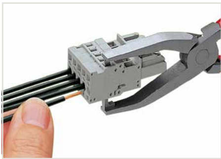
Operating tool Inserting a conductor – side-entry wiring (example shows a female plug). With ferruled conductors, it is necessary to use a terminal block one size smaller than the conductor's nominal cross section.
