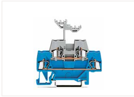
Double-deck terminal blocks accommodate two circuits of different potentials on two decks; different circuits can be differentiated by color coding either deck (280 Series). The lower deck is wider than the upper for ease of wiring.
