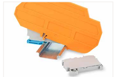
Ex e II/Ex i terminal strip Notice: The movable feet of terminal blocks and separator plates must face the same direction.
