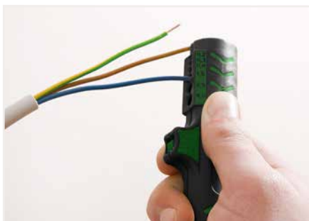
Stripping a wire insulation.
