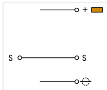
Actuator terminal block; with shield connection
