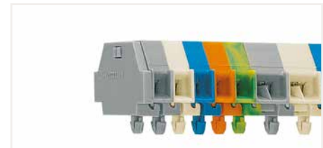
Terminal strip; with snap-in mounting feet; for 0.6 ... 1.2 mm plate thickness; 3.5 mm mounting hole diameter (also for 210-154 Aluminum Rail or with 209-120 Mounting Foot for DIN-35 rail)
