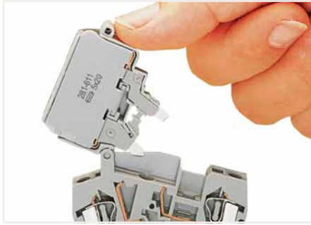
Fuse replacement: Before replacing a fuse, pivot the fuse holder into the locked open position.
