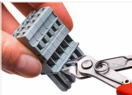
Coding a female plug by removing coding finger(s) via cutting tool. Do not remove the first and last coding fingers or use an additional locking lever.
