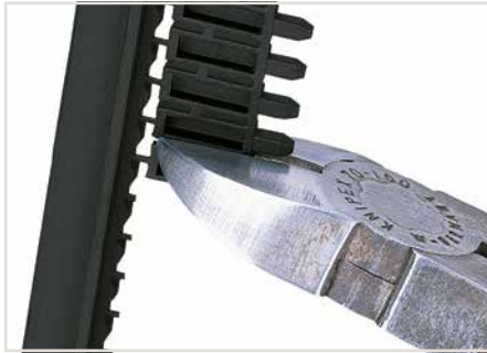
Remove unrequired areas from the sidewalls.
