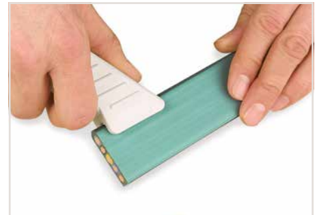
Cut both flat cable insulation sides via stripping knife.
