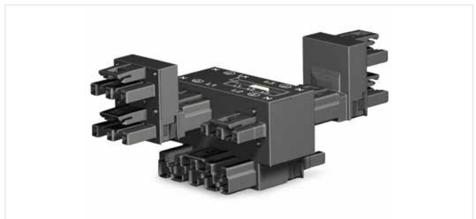
Additional h-distribution connectors double L1 and L3. This results in the following connection option: L1/L1/L2/L2/L3/L3 with jumper in position L2
