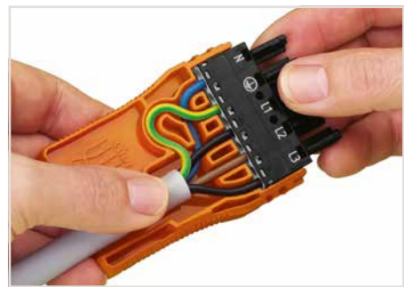
Strip conductor ends to a length of 9 mm (see marking). Slide connector to the stop over conductor ends.
