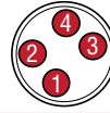
Input voltage, male, 4-pin (M8) integral connector pin-out as viewed from the end of the sensor
