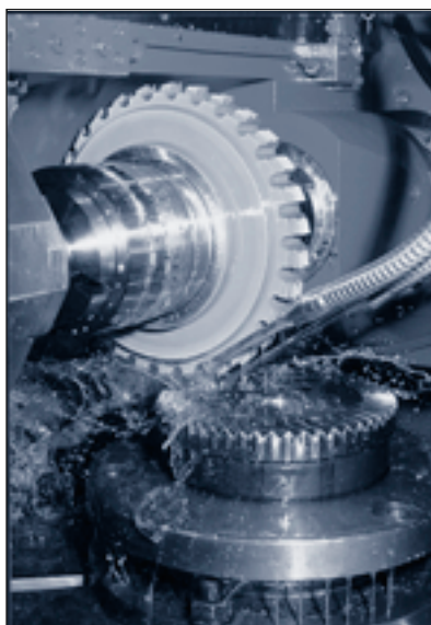
CNC Machining of a PowerTRUE* right angle gear
