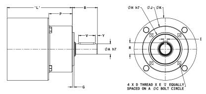
\* 'L' Dimension will change depending on motor being used. Note: Mounting adapters available for both round and square motors.
