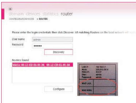
The configuration of the C6 Router is protected with necessary log-on data.
