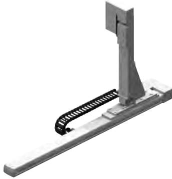
Wiring 1 with cable track
