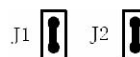
(d) J1 short circuit, J2 short circuit CW/CCW mode and effective at downward-falling edge
