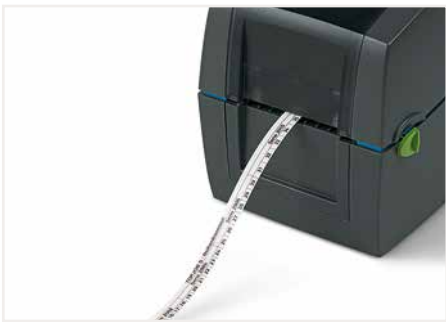
Printing a marking strip (2009-110) via Smart Printer.
