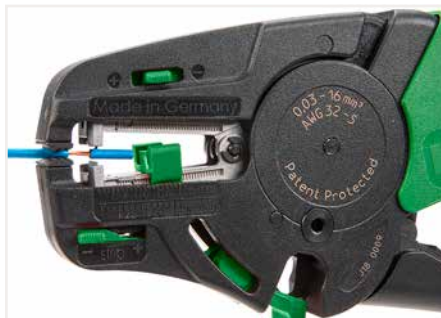
Partially stripping a conductor.
