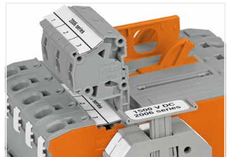
Alternatively, measurement can also be performed using Connector (2006-511) from terminal block 1 to 2. Spacer modules (2006-549) must be used to compensate for the 15 mm terminal block width.
