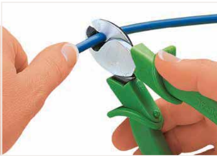
Cutting a cable.
