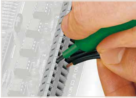
Inserting a conductor via 3.5 mm screwdriver. Screwdriver actuation parallel to conductor entry.
