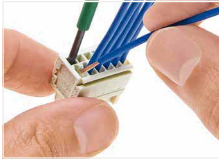
Inserting a conductor via (2.5 x 0.4) mm screwdriver – CAGE CLAMP® actuation parallel to conductor entry.
