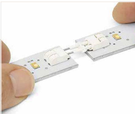
Assembly: Place PCBs on a flat surface and connect terminal blocks on adjoining PCBs via board-to-board link. Disassembly: Pull PCBs apart (max. 10 mating cycles).
