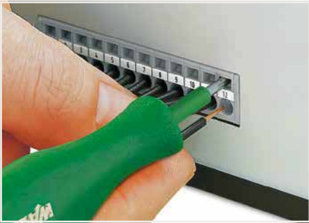
Feedthrough PCB terminal strips – front-entry conductor termination
