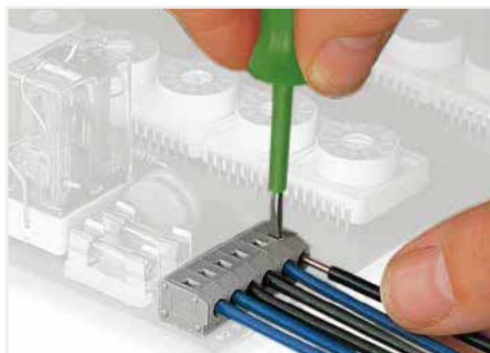
Removing conductor via (2.5 x 0.4) mm screwdriver.
