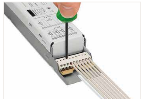
Removing a conductor via 1.0 mm Ø disconnection tool (206-B40).
