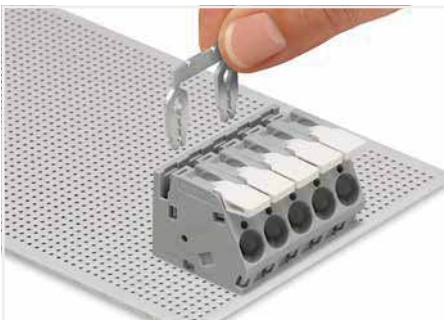
Insert the comb-style jumper bar.
