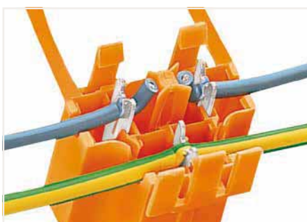
Snapping socket halves together will automatically cut and terminate a "live" conductor without stripping – enables switching applications (e.g., door switches).
