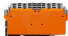
Terminal block for pluggable modules; 12-pole; with 4-conductor terminal blocks; with marker carrier; with orange separator; for 35 x 15 mm and 35 x 7.5 mm DIN-rails; 2.5 mm 2
