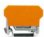
Terminal block for pluggable modules; 6-pole; with 2-conductor terminal blocks; with orange separator; for 35 x 15 mm and 35 x 7.5 mm DIN-rails; 2.5 mm 2
