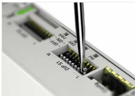
Configuration via DIP switch
