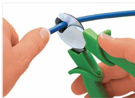
Cutting a cable.
