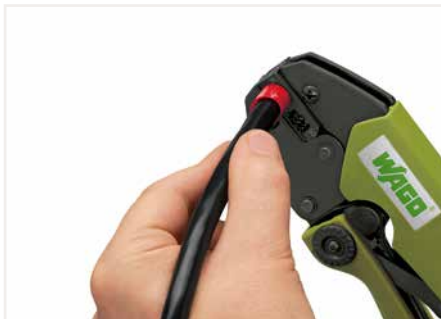
Squeeze handles until ratchet mechanism is released.
