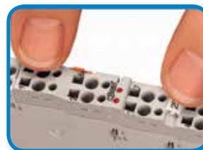
Place the connector into the I/O module
