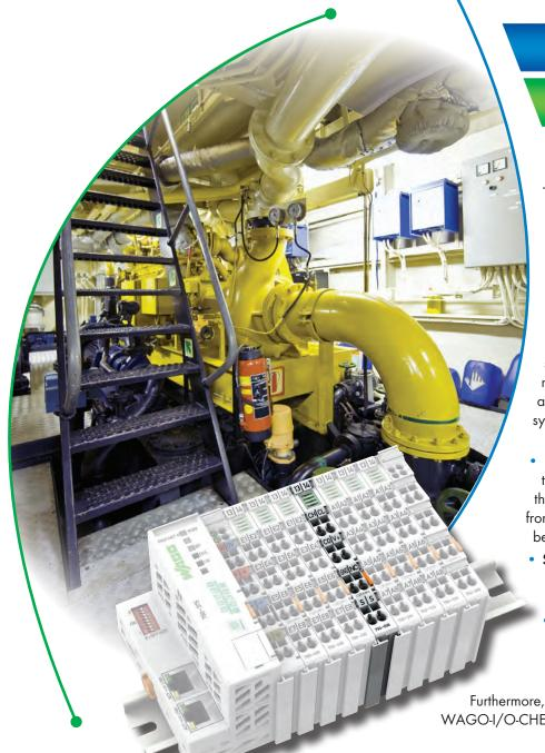
The compact, 12mm wide CAN gateway module provides a link between CAN networks and other popular fieldbuses such as MODBUS, EtherNet/IP, Profinet, and more. Supporting both the CAN 11 bit and 29 bit identifier protocols, this module can be configured as a CANopen or SAE J1939 master/slave within a WAGO-I/O-SYSTEM node. Three operating modes offer additional flexibility for your control system strategy.
