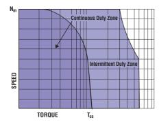
**NOTE:** Continuous torque specifications obtained with motor mounted to an 8.5"x12"x 0.25" aluminum plate at 25°C ambient. Typical values are within  $\pm$ 10% of rating.
