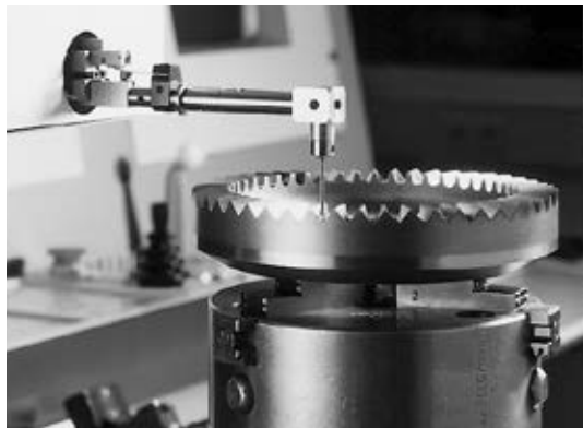
Computerized mapping of gear tooth profile
