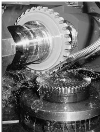
CNC machining of a PowerTRUE right-angle gear
