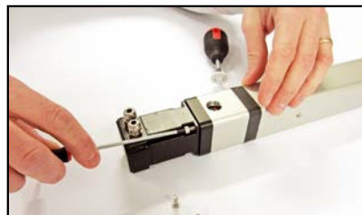
Tighten motor mounting screws
