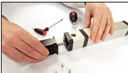
Insert motor shaft into coupling
