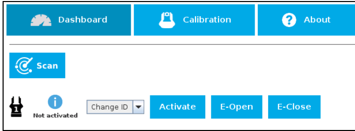
Fig. 3-5: Activating a gripper and assigning an ID.
