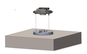
Slide bottom shield/magnet assembly over shaft and lock alignment pins into adapter plate. Push down bottom shield all the way so it lies flat on the adapter plate.
