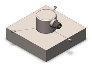
Secure housing by tightening the three M2.5 screws using a Philips screw driver with a torque of 0.4 Nm
