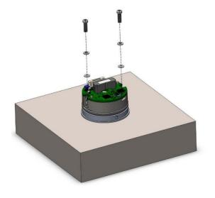
Insert two M2 screws with washers and lock washers and tighten using a Torx T6 key with a torque of 0.25 Nm.
