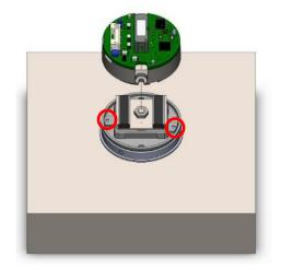
The alignment pin geometry is not symmetrical as shown by the red circles. Take care not to damage the pins during installation onto the adapter plate.
