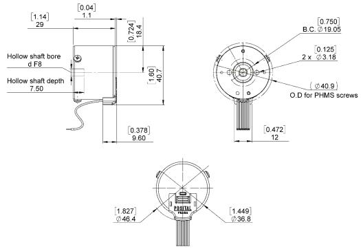
E5xU-PRQ: d = Ø4mm, Ø5mm, Ø6mm or Ø1/4"
