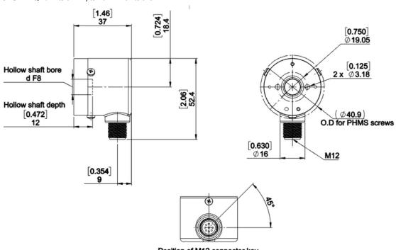
Position of M12 connector key
