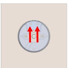
For a correct flange orientation, notice the two holes shown in the image. The connector location should be always assembled relative to these two holes.
