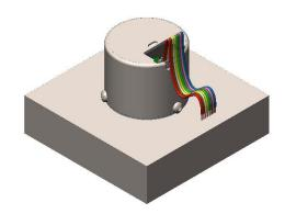
Connect cable assembly to the PCB by plugging the connector into the PCB.
