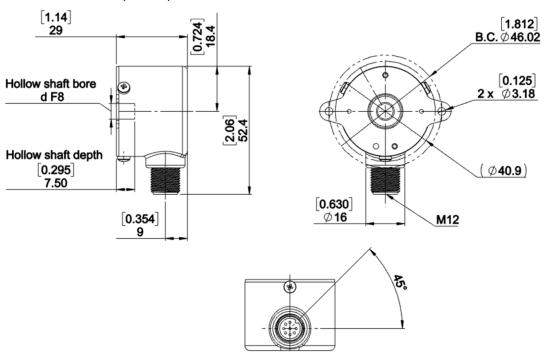
Position of M12 connector key
