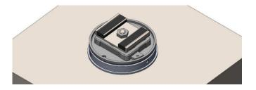
Align magnet with plastic frame on the bottom shield.
