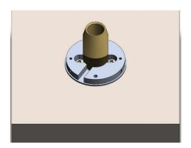
Tighten mounting screws while pushing down on the centering tool and remove centering tool. Tighten screw to a typical torque of 0.4 Nm (Actual torque value may change due to machine screw selected and base mounting material)
