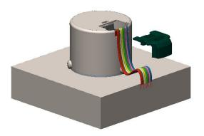
Assemble the cable clip onto the metal housing to secure the cable assembly.
