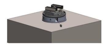
Tighten both set screws with a 1.3mm [0.05"] hex key, using the channel hole in the adapter plate with a torque of 0.5 Nm.
