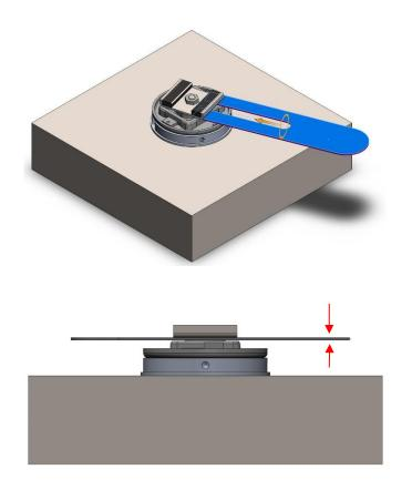
Slide gapping tool (Required thickness of 0.7mm [0.0275"]) between magnet and bottom shield. Push magnet down.
