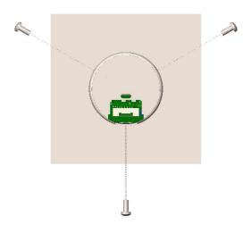
Slide housing over adapter plate. Secure housing by tightening the three M2.5 screws using a Philips screw driver with a torque of 0.4 Nm
