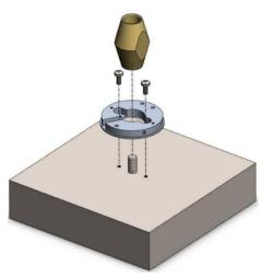
Slip adapter plate over shaft and use screws, depending on tapped holes in motor frame, to secure. Slip centering tool over shaft to center adapter plate to the shaft centerline.
