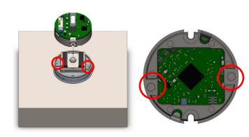
Align PCB with carrier to frame (two different keys) and push down until it locks into place.
