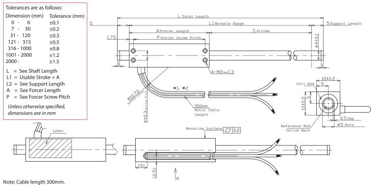
The bending radius of the motor cable should be 10.72 mm (wire diameter 1.34 \* 8) as suggested by the wire manufacturer. This radius should be maintained. Use supplied connector to attach the proper high-flex cable as required by your application.
