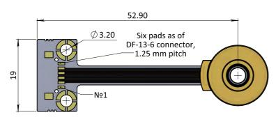
Encoder with flexible connector bus (bottom view).
