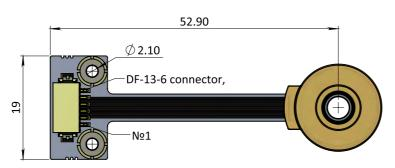
Encoder with flexible connector bus (bottom view).
