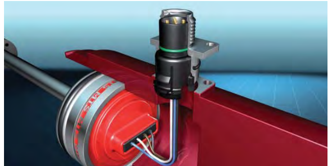
Figure 8. The connector insert is taken out of the cylinder through a bore hole. The flange housing can be snapped into position easily from outside.
