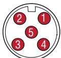
Integral D34 connector (male) as viewed from the end of the sensor
