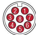
Integral D84 connector (male) as viewed from the end of the sensor
