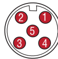
Integral D34 connector (male) as viewed from the end of the sensor
