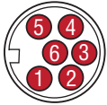
Male, 6-pin (D60) integral connector pin-out as viewed from the end of the sensor
