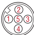
Female, 5-pin (D54) integral connector pin-out as viewed from the end of the sensor
