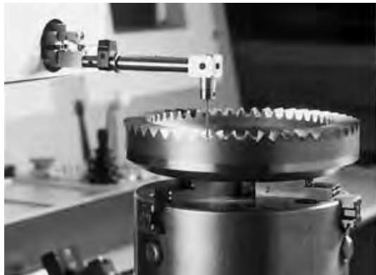
Computerized mapping of gear tooth profile
