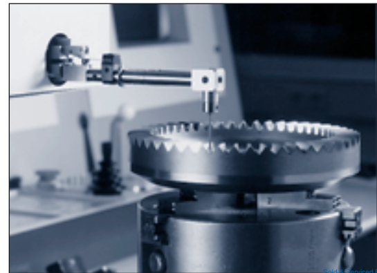
Computerized mapping of gear tooth profile
