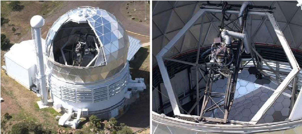
Figure 3: The Hobby-Eberly Telescope (left) with its dome open. On the right is a close-up of the HET with the primary mirror and telescope structure, incl. the tracker that supports the PFIP. © 2012 HET
