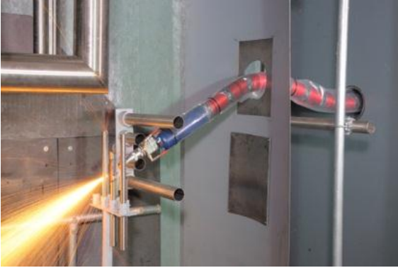
Figure 4: The laser tool of the snake-arm robot can cut through steel like butter. © 2012 OC Robotics
