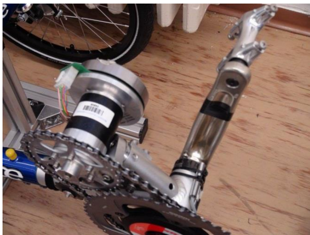
Figure 3: The 90 W flat motor used in the recumbent trike provides enough power for the drive task. © 2012 IRPT
