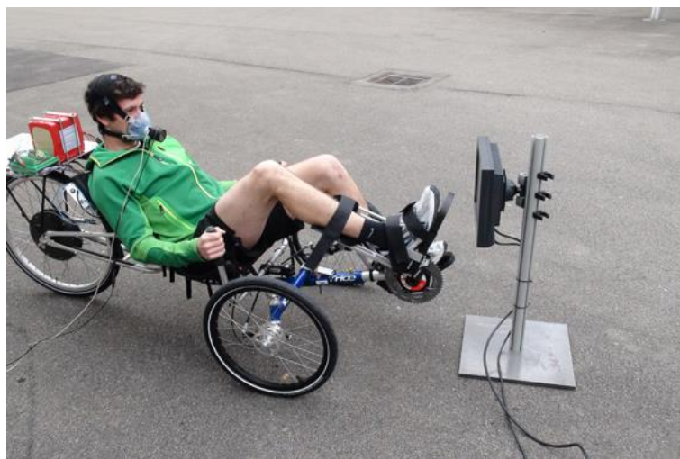
Figure 2: Recumbent trike prototype for adults. The power for the flat motor and rear wheel hub is supplied by a battery (red battery pack). © 2012 IRPT
