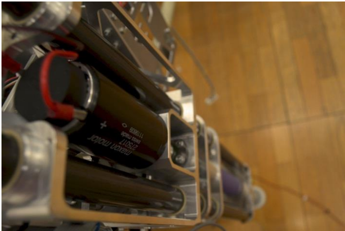
Figure 3: maxon View on DC RE40-Motor © 2011 ETH Zürich
