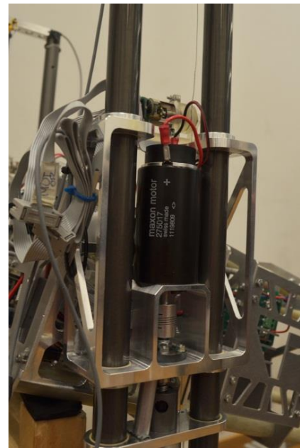
Figure 5: The maxon DC RE40 motor in the leg module takes care of the jump motion. © 2011 ETH Zürich
