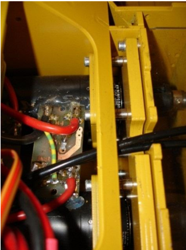
Figure 5: The model loader is driven by 150 W maxon DC motors mounted below it. Photo: Marcel Sigrist
