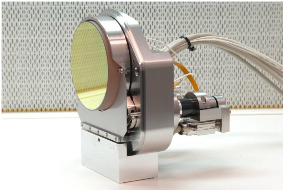
Figure 4: The first prototype of the FSM, standing upright on the laboratory table. © 2011 SPIE Optics & Photonics/TNO
