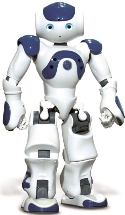
Nao, Romeo's smaller brother. His shoulders are equipped with maxon DCX motors. Image © Aldebaran
