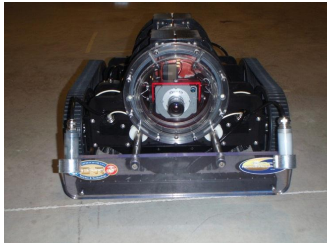
Figure 3: This close-up of the HullBUG clearly shows its sensor alignment system that helps it keep on course while cleaning a hull. © 2011 SeaRobotics
