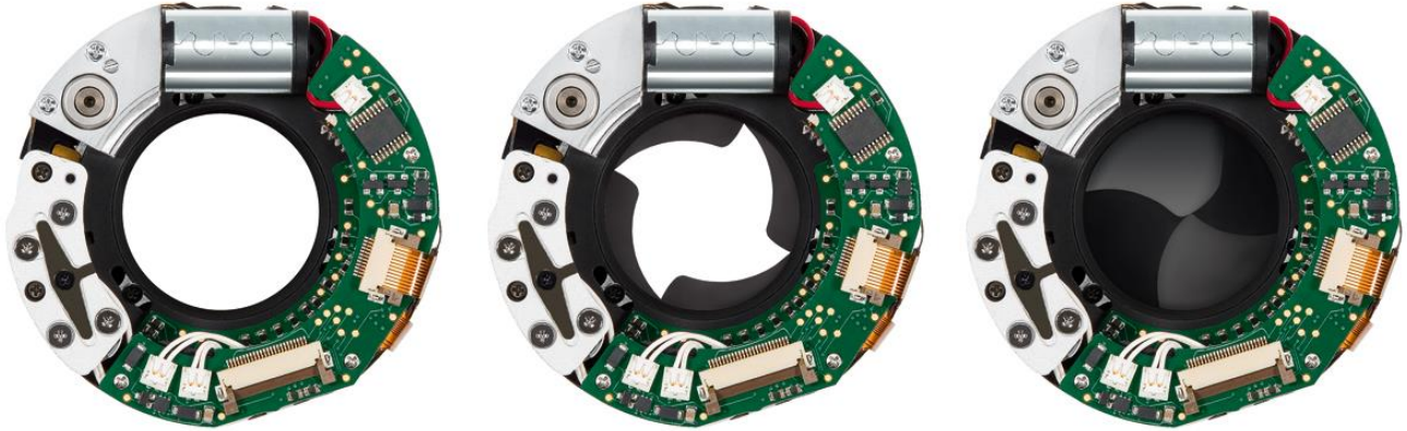
Figure 2: The central shutter generates no vibration and is very fast. The gear motor is used for tensioning three springs that store the energy for the central shutter.
