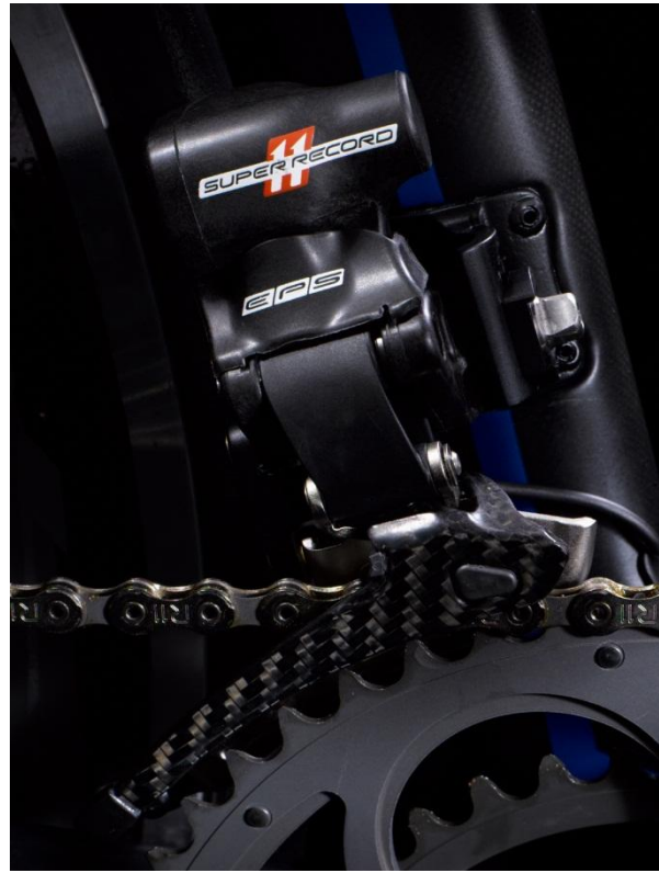
Figure 3: The Campagnolo Super Record® EPS is the lightest shift system in the world that is largely made of carbon. ©2012 Campagnolo
