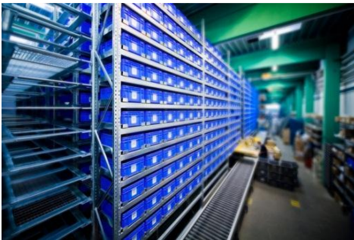
Figure 5: An automated storage and retrieval system makes sense in warehouses with more than 1000 storing positions. The shelves are modular and based on a conventional pallet rack. © 2012 YLOG
