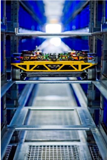
Figure 2: The shuttles, which weigh approx. 50 kg, need very little space for maneuvering.
