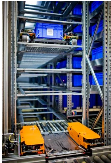
Figure 6: Up to 500 transport vehicles can be driving around in a warehouse. © 2012 YLOG
