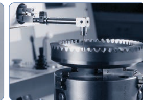
Computerized mapping of gear tooth profile
