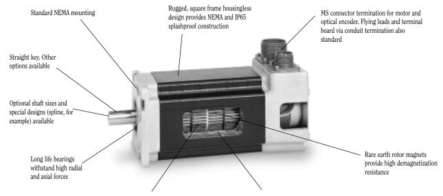
Large diameter rotor coupled with optimum magnetic design produces highest torque and acceleration - both N and K Series Sigmax® technology in K Series adds flux concentrating rare earth stator magnets for even higher torque and acceleration than N series
