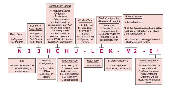
The example model number above indicates a N series standard NEMA 34 frame motor with a three stack rotor. This motor is equipped with a heavy duty front end bell and shaft, and a sealed system rear end bell with MS connectors. It also has a bipolar parallel connection, a J winding, a straight keyway, encoder mounting options and a shaft seal.
