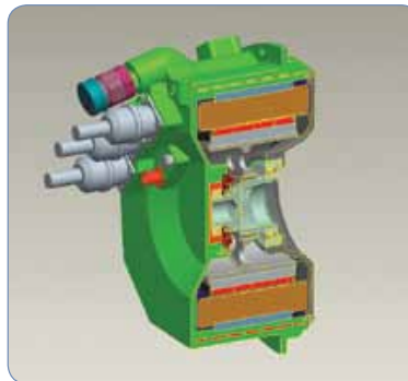
200 kW electric starter/generator
