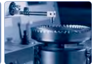
Computerized mapping of gear tooth profile
