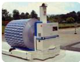
World's first laser-guided vehicle Tetra Pak, Singapore, 1990
