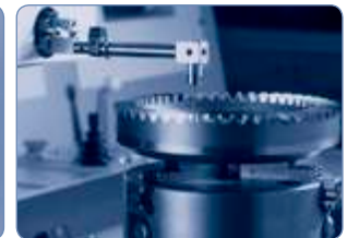
Computerized mapping of gear tooth profile
