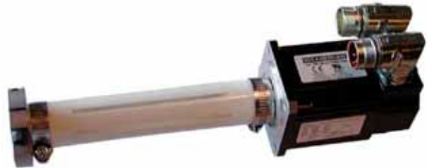
Figure 6. Compliant coupling and load used in servo comparison tests.
