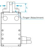
\* The gripping force of the GRSS is measured with the finger attached.
